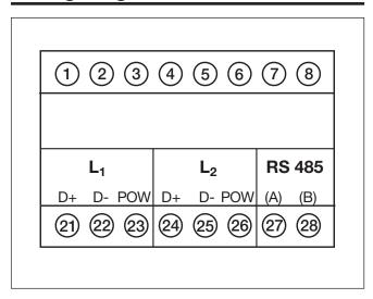
Use 3\*1,5mm2 single core wire for  $L_1$  and  $L_2$  bus Use 2 wires with shield for the RS485 connection (Distance up to 1200 Meter)
